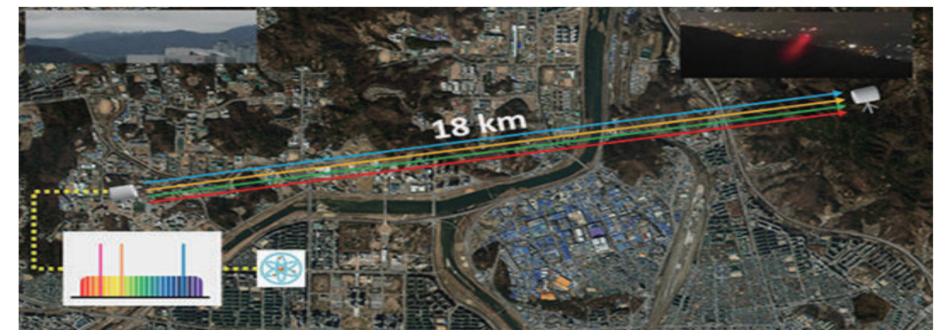
Figure 1] Phase-coherent transfer of comb-rooted optical frequencies over an 18-km free space link.
